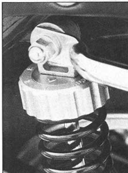
Damping that's four-way adjustable
